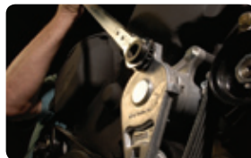
Serpentine Ratcheting Wrench Set Facilitates the speedy release of tension on serpentine belt drives.
